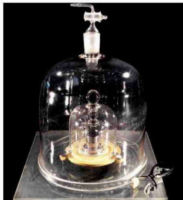
Kilogram standard serving as an international reference kept at the International Bureau of Weights and Measures in Sèvres (under several Russian doll bells).
